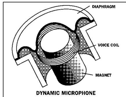
Dynamic microphones have relatively simple construction and are therefore economical and rugged. They can provide excellent sound quality and good specifications in all areas of microphone performance. In particular, they can handle extremely high sound levels: it is almost impossible to overload a dynamic microphone. In addition, dynamic microphones are relatively unaffected by extremes of temperature or humidity. Dynamics are the type most widely used in general sound reinforcement.
