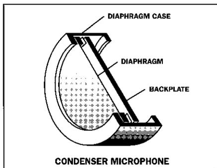
The construction of a condenser microphone must include some provision for maintaining the electrical charge or *polarizing* voltage. An *electret* condenser microphone has a permanent charge, maintained by a special material deposited on the backplate or on the diaphragm. Non-electret types are charged (polarized) by means of an external power source. The majority of condenser microphones for sound reinforcement are of the electret type.
