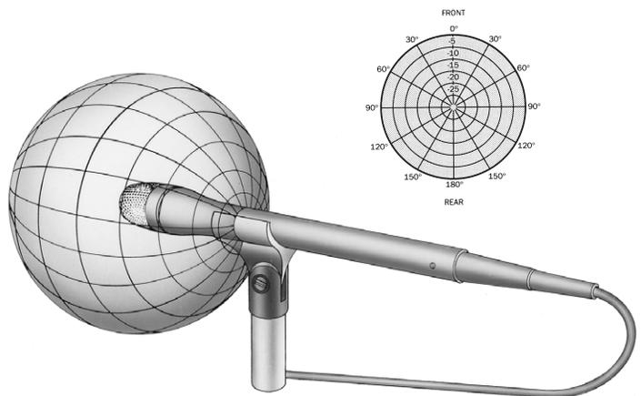
The **unidirectional** microphone is most sensitive to sound arriving from one particular direction and is less sensitive at other directions. The most common type is a cardioid (heart-shaped) response. This has the most sensitivity at 0 degrees (on-axis) and is least sensitive at 180
